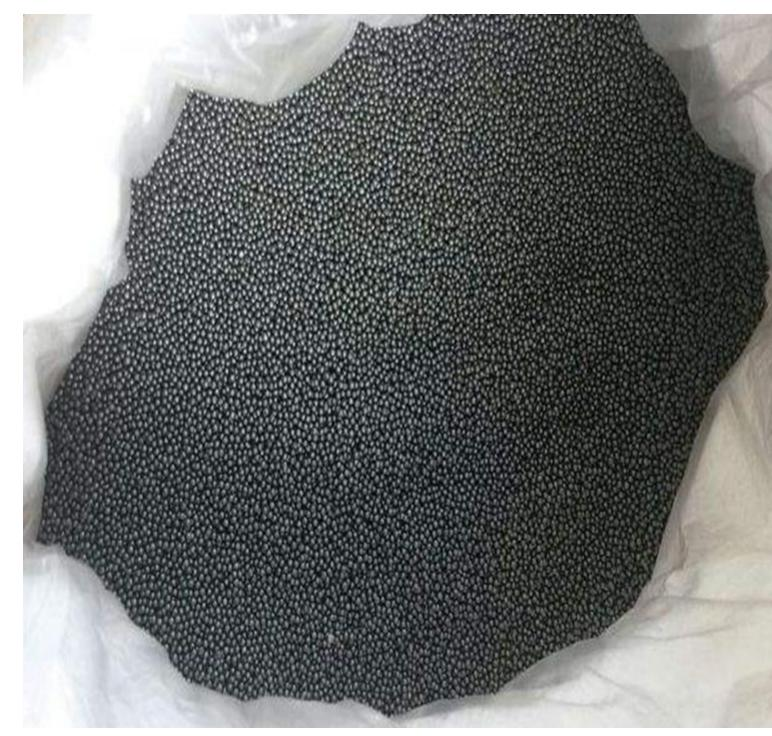
Stainless steel shot is also available. It is made of stainless steel and is widely used in industries that abrasive cleaning. The high hardness of S390 steel makes it the ideal shot for hard-to-treat materials commonly used in die-cast products, zinc, and aluminium. Its durability and long life make it a great of avariety of applications.
