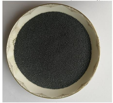
Carbon steel cut wire shot is a commonly used blasting media. Its fine grain size and higher hardness a better choice for components that need a high level of blasting media harness. It can also be recycl multiple times. This makes it a valuable material for many peening applications. Once used, cut wire s recyclable and can reduce the cost of steel blasting operations. If you want to increase the life of your stainless steel parts, this is the best choice for you.
