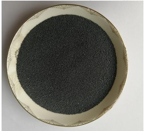
Carbon steel cut wire shot is a commonly used blasting media. Its fine grain size and higher hardness a better choice for components that need a high level of blasting media harness. It can also be recycl
