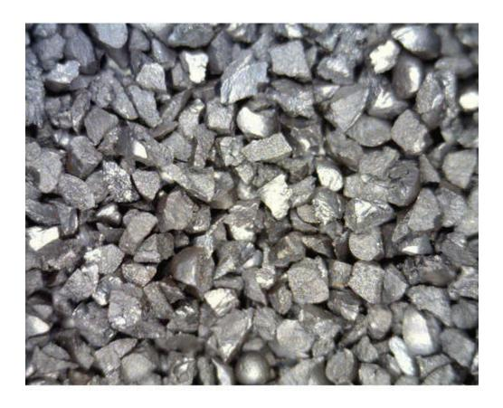
Steel grit is an abrasive, made of small, randomly shaped particles that can be sifted out easily. Its high hardness makes it useful for descaling steel components and removing sand from castings. The procestraightforward, and Composition Materials supply a variety of hardness grades. You can choose from or HRC, depending on the desired degree of aggressiveness. Regardless of the type of abrasive you can it's worth looking into.
