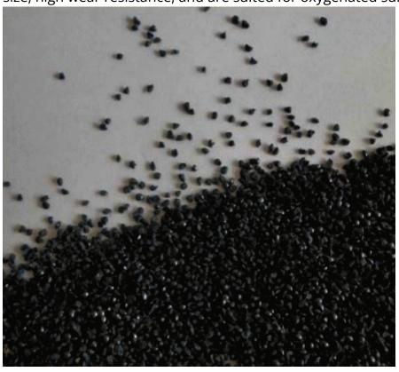
The steel grit g40 from China is produced by atomizing molten steel and thermal treatment. GH grits are 60-66 HRC and are especially suited for finishing and cutting stone and granite. GH grits are available in a wide range of sizes and hardness.
