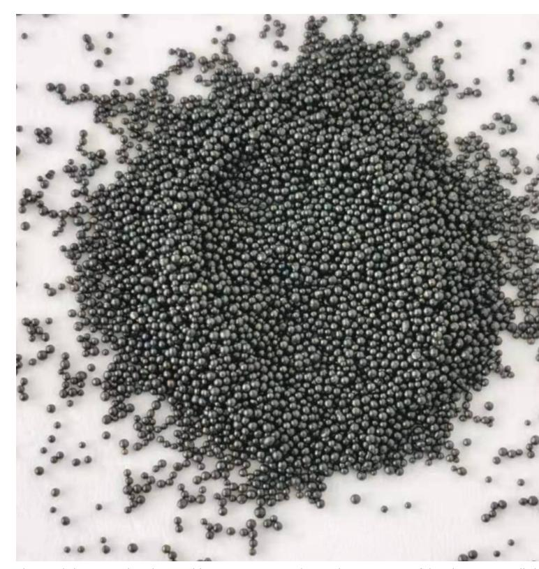
This steel shot is used in abrasive blasting processes. The steel composition of this shot is generally he carbon and low in manganese. It meets SAE hardness specifications both as-cast and after additional tempering. It is manufactured by a company that uses advanced technology. It is suitable for a wide applications. It can be easily shaped to meet the required requirements.
