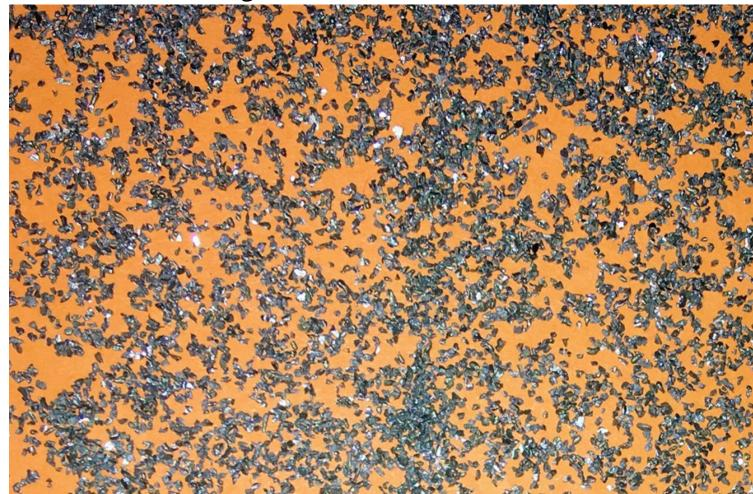
There are many types of abrasives, but one of the most common is steel grit. This type of abrasive has randomly shaped grain and varies in hardness. It will erode and etch surfaces, depending on the appoint is available in a wide range of sizes, from coarse to very fine. The size of the particles will determine of abrasive used.
