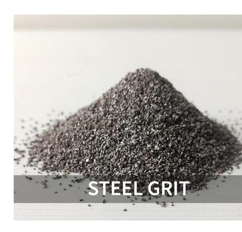
A steel grit is an abrasive material that is made by crushing and screening abrasive materials, and the tempering them to a desired hardness. The abrasive particles in steel grit are often very sharp, and a for cleaning and smoothing surfaces in blasting. They come in many shapes and sizes, and are used tremove various degrees of coatings and rust.
